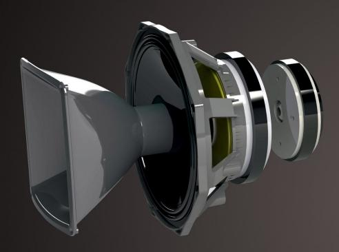
The core of the IsoWave system consists of 12" extremely Low-Mid driver with a coaxially mounted 1.4" exit compression driver. The high frequency driver is loaded with a 90° horizontal x 60° vertical waveguide. This sophisticated waveguide also loads the 12" low frequency driver. Together the system forms a high sensitivity, high SPL motor system with exceptional linearity and directivity control.
